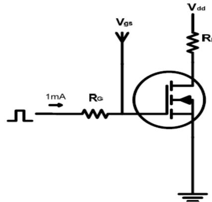
**Switch Time Test Circuit:**
