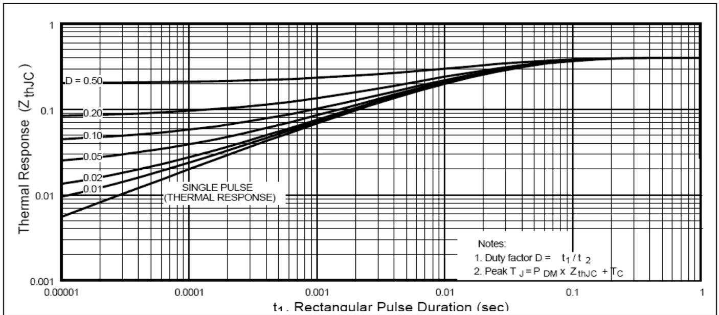
Figure 7. Maximum Effective Transient Thermal Impedance, Junction-to-Case
