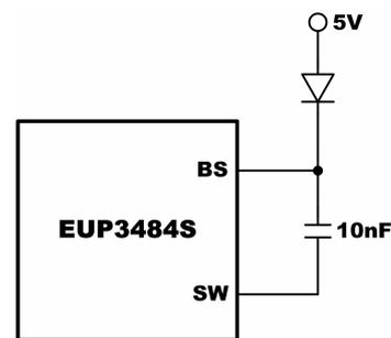
**Figure 3. Add Optional External Bootstrap Diode to Enhance**
